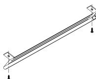
Step 2 Secure the brackets to the mounting surface by using two tapping screws
